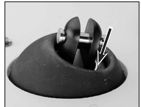
Clean drum bearings.
