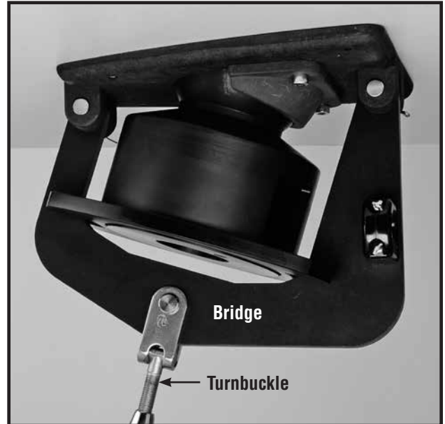
Turnbuckle to bridge
